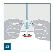
Grasp the tabs of the sheath. While holding the catheter in place, pull the tabs outward simultaneously to peel the sheath from the catheter.
