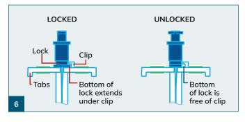
Check that the dilator is locked within the introducer sheath to prevent separation of the two components during insertion. To lock the dilator, rotate the dilator so that the flange on its hub locks under the clip on the sheath.
